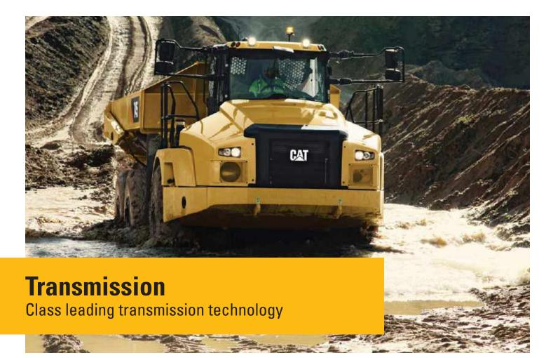
The Cat High Density Power Shift (HDPS) nine-speed forward, two-speed reverse transmission, designed specifically for Articulated Trucks, features Advanced Productivity Electronic Control Strategy (APECS) and Electronic Clutch Pressure Control (ECPC) that deliver smooth gear changes with improved acceleration and higher productivity.
