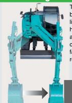
This feature prevents damage to walls. beams and buried structures by limiting the depth, height, and lefthanded offset value reached by the attachment. It both prevents unwanted contact with external objects and facilitates side-wall digging and other repetitive operations.
