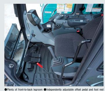
excellent visibility OLarge travel pedal New reclining seat can be lowered well down to
