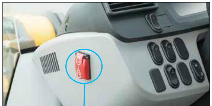
Engine shutdown secondary switch
