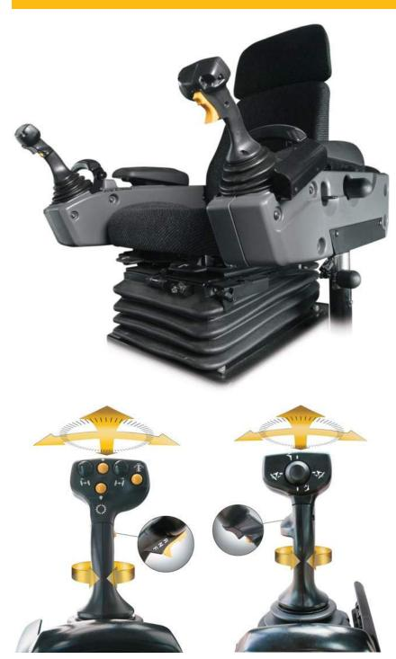
Operators are more comfortable and productive with two electro-hydraulic joysticks. New and experienced operators around the world report that the controls are easy to learn, and that the new electronically adjustable control pods make it easier to position them for optimal comfort, visibility and proper operation.
