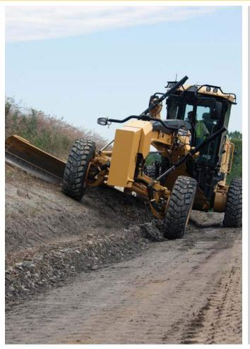
If you work in soft underfoot conditions where traction can be a challenge, optional All Wheel Drive (AWD) can give you the additional power to the ground you need to work more efficiently in mud, gravel, sand or snow. The added traction helps reduce sliding on side slopes.
