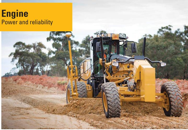
Cat C7 and C9 engines give you the performance you need to maintain consistent grading speeds for maximum productivity. Superior torque and lugging capability provide the power to pull through sudden, short-term increases in loads.
