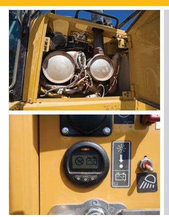
Emissions reduction technology is designed to be transparent – regeneration runs automatically in the background while you work. Diesel Exhaust Fluid (DEF) can be conveniently refilled when you refuel.
