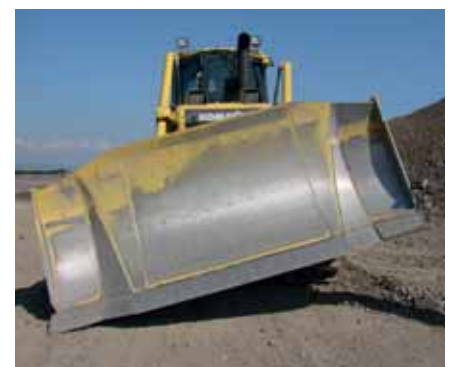
Hydraulically adjustable tilt: 870 mm
