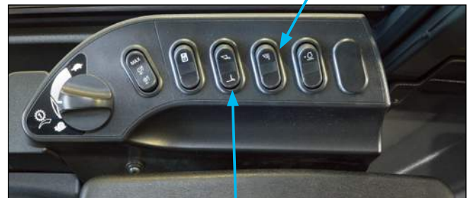
Attachment selector switch
